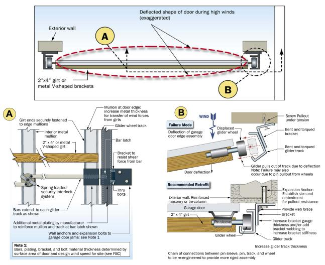
Figure 3.2.5. Recommended details for upgrading garage doors.
