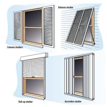
Figure 3.2.8. Examples of storm shutter styles.
